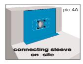
1.4 DN 70: Unfold the preassembled connecting sleeve and glue to parapet and slab (picture 4). DN 50: Punch 14mm holes for the bolts into the connecting sleeve. Use the loose flange to indicate the position of the holes.
